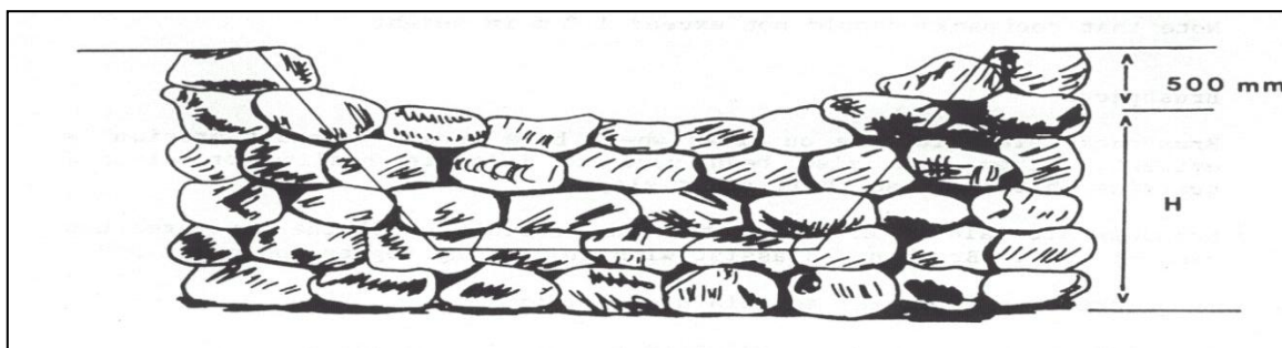
Fig. 2. Details of typical stone pack – Rocks should be elongated/flat/oval-shaped and hard durable and heavy – Pack the rocks so the long axis lies parallel to the upstream slope of the structure (1.5:1) – Ensure good bond in length and depth of structure with foundation and shoulders.
